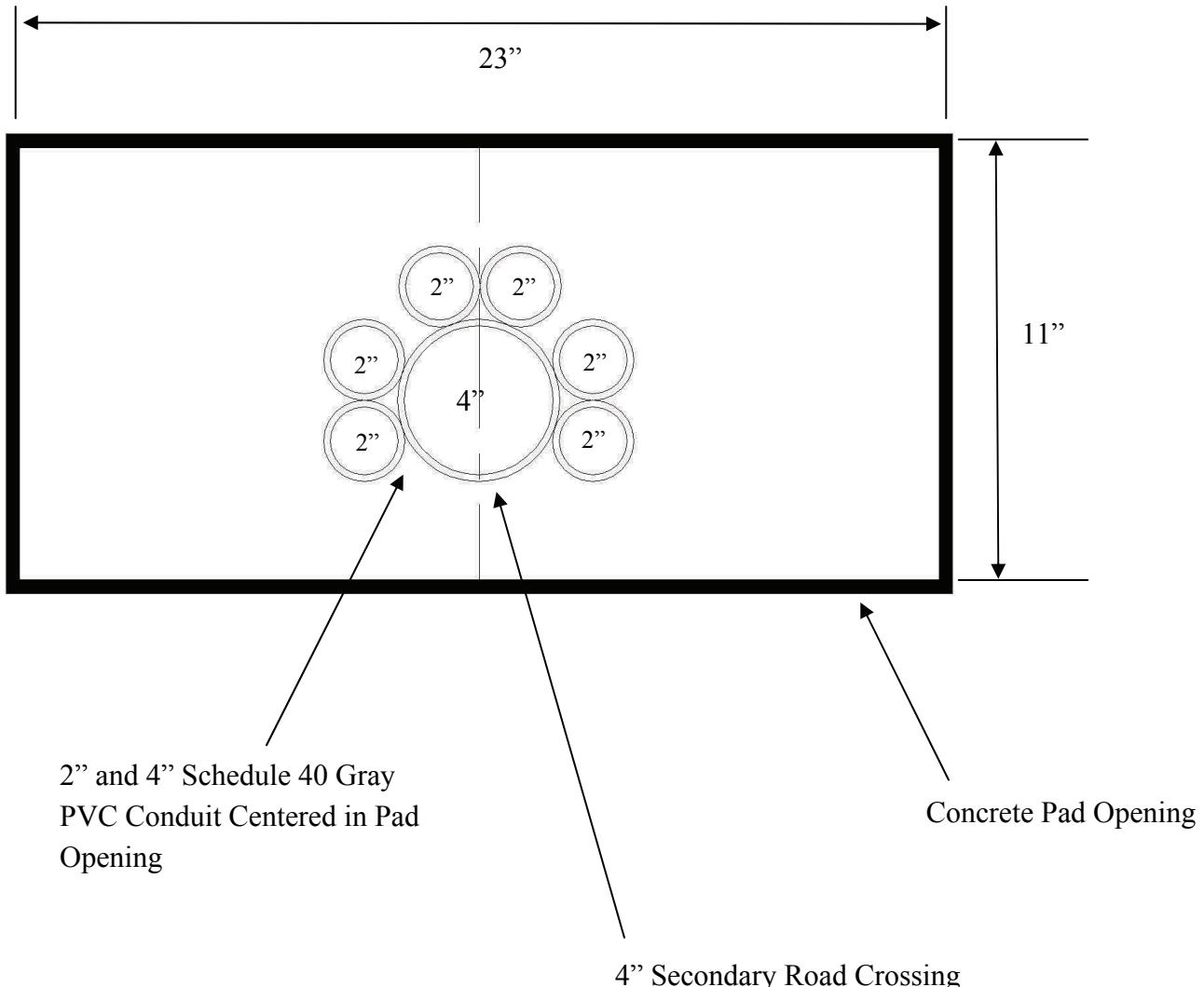
Conduit sizes may vary with design. If conduit number and size are different than as shown, please contact KUA's conduit inspector.
