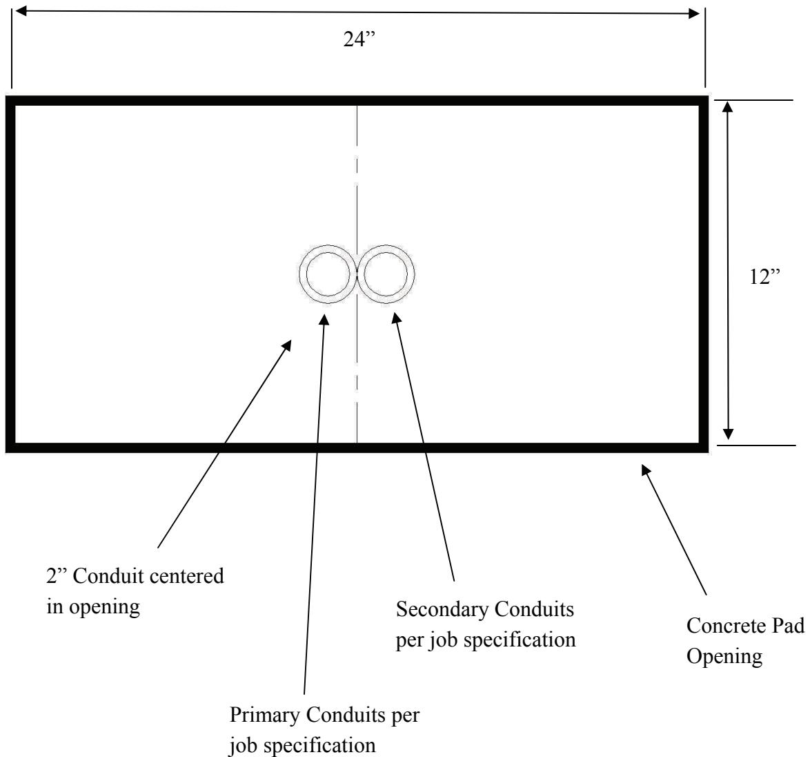
Conduit sizes may vary with design. If conduit number and size are different than as shown, please contact KUA's conduit inspector.
