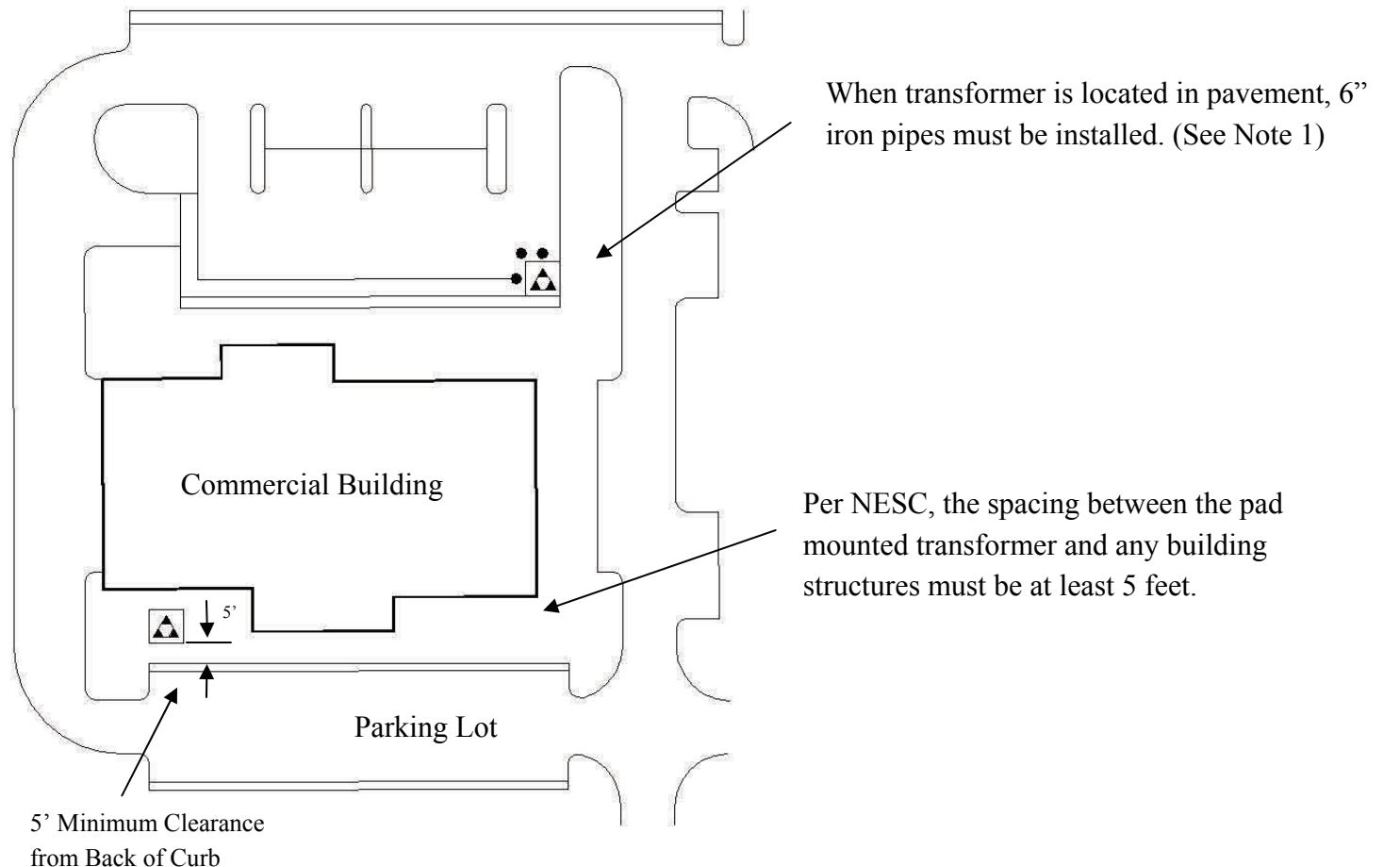
**Protection of Transformers and Junction Boxes:** The transformer and/or junction box shall be protected by the following means:
