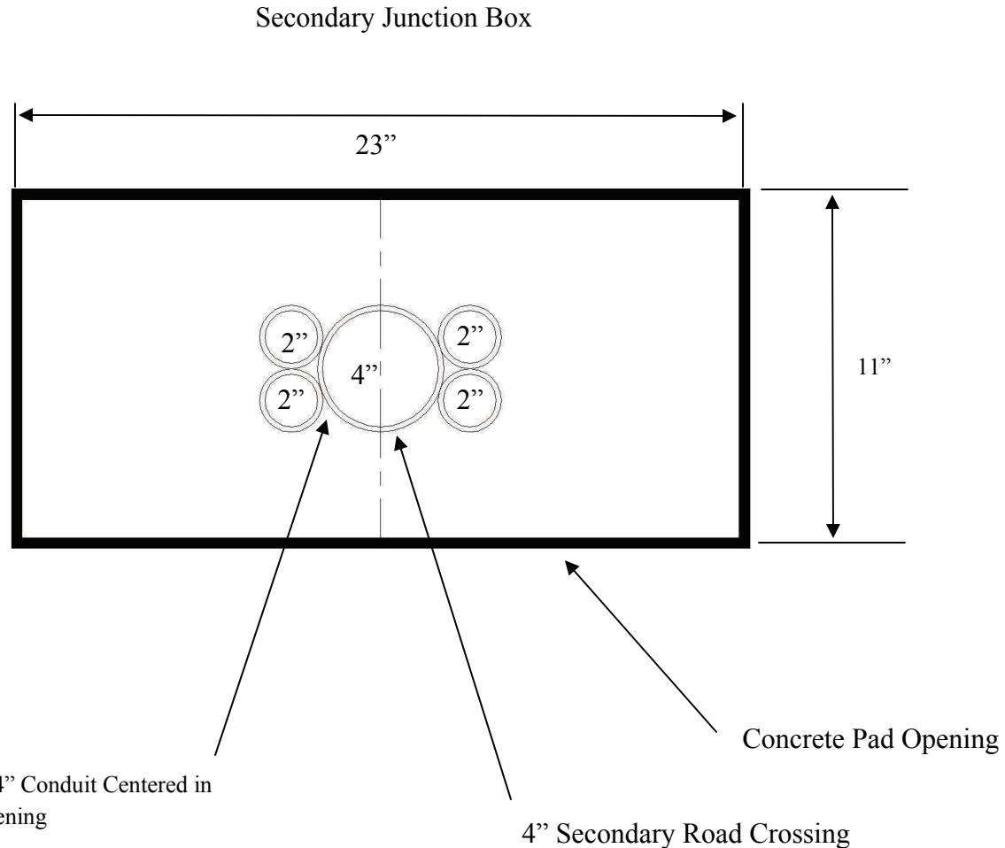
Conduit sizes may vary with design. If conduit number and size are different than shown, please contact KUA's conduit inspector.
