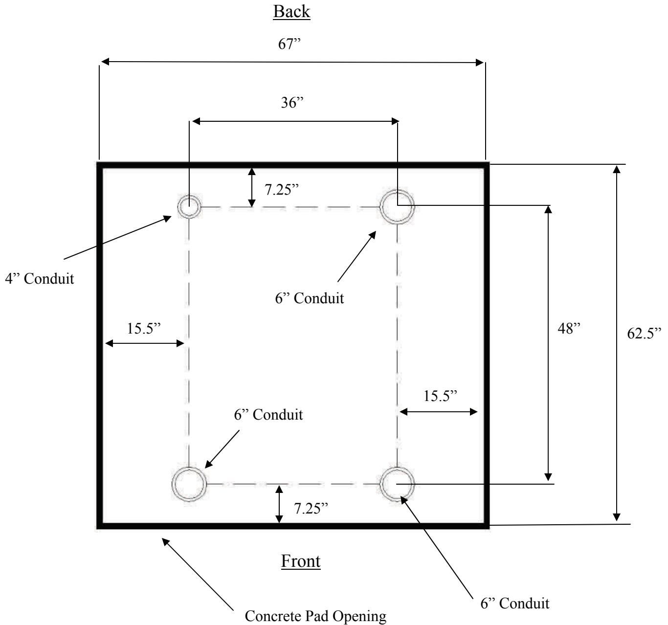
Conduit sizes may vary with design. If conduit number and size are different, please contact KUA's conduit inspector.
