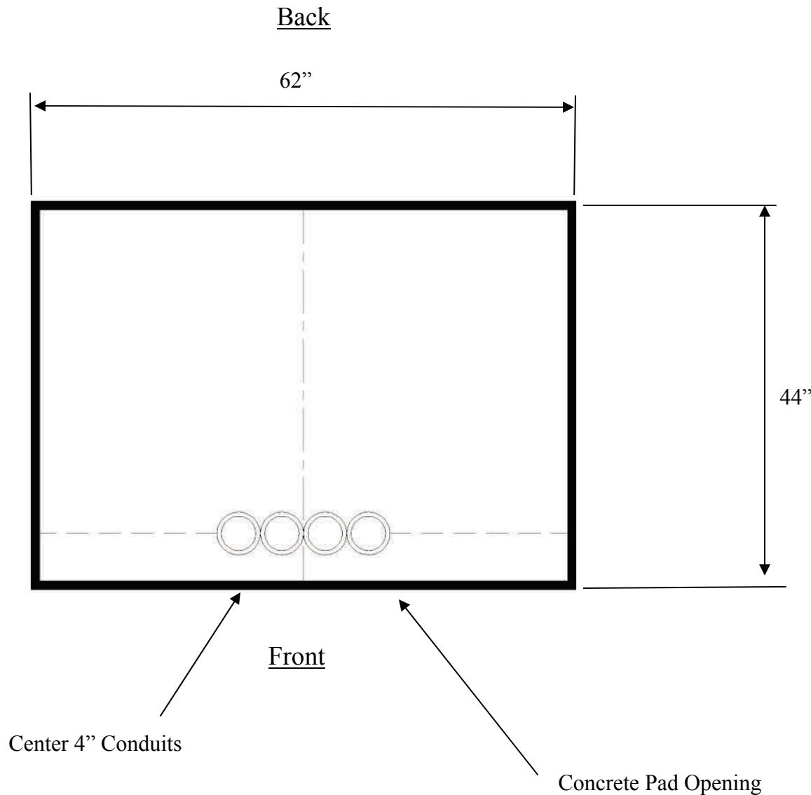
Conduit sizes may vary with design. If conduit number and size are different, please contact KUA's conduit inspector.
