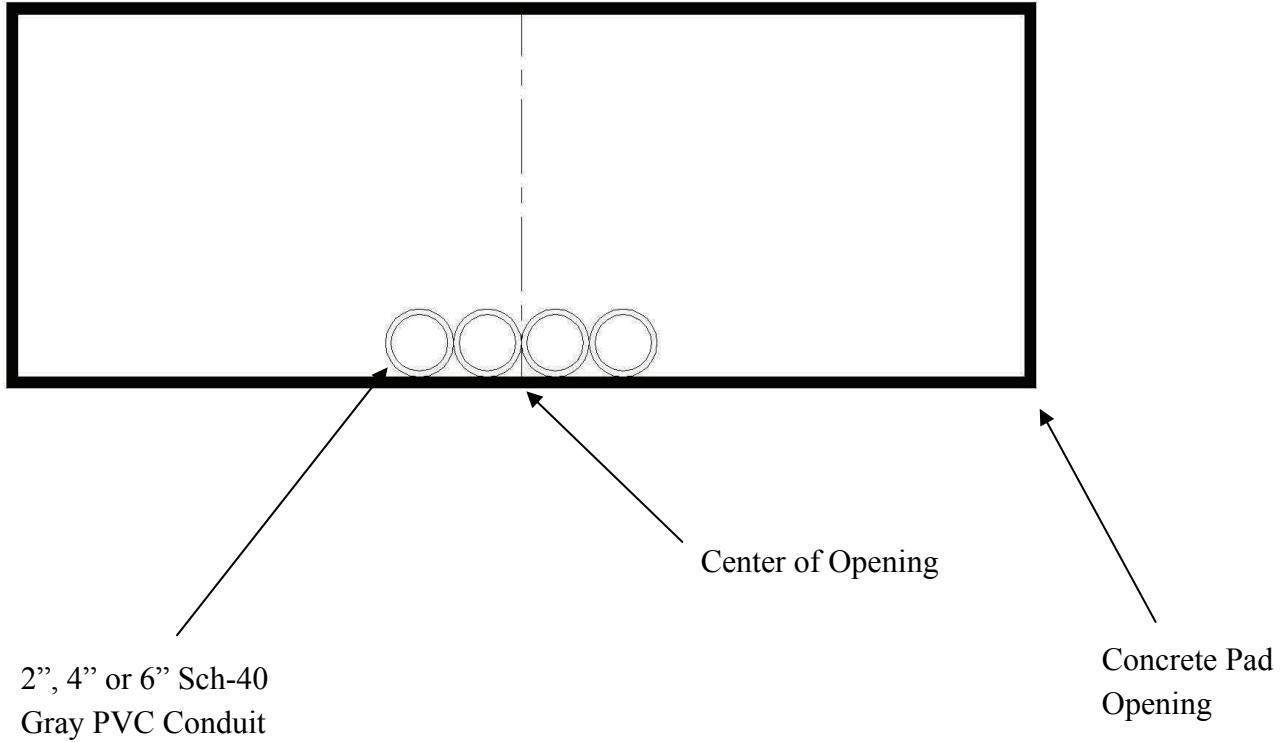
Conduit sizes may vary with design. If conduit number and size are different than as shown, please contact KUA's Conduit Inspector.
