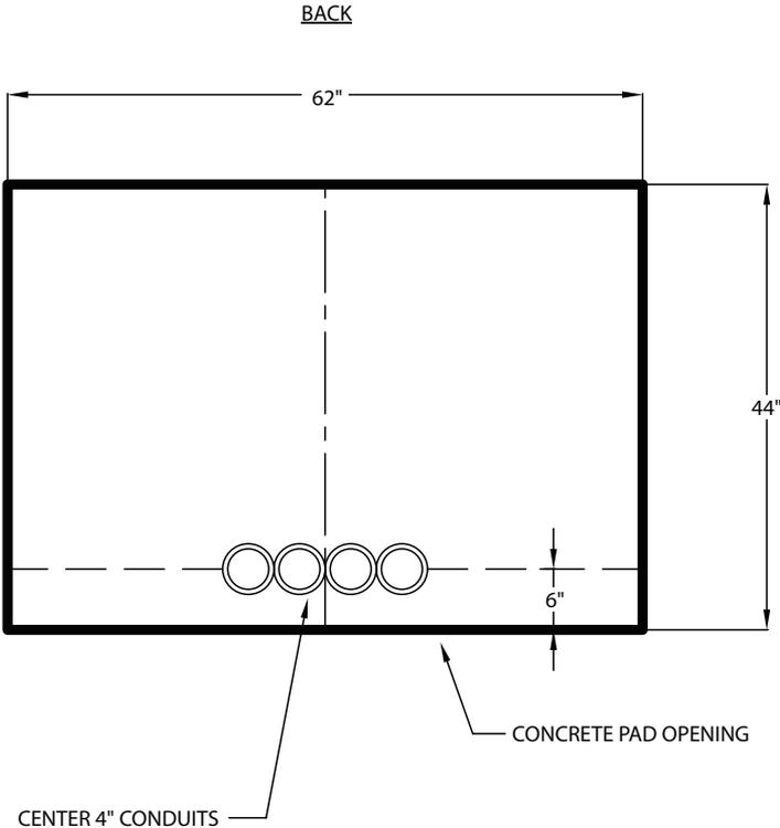
Conduit sizes may vary with design. If conduit number and size are different than as shown, please contact KUA's Conduit Inspector.
