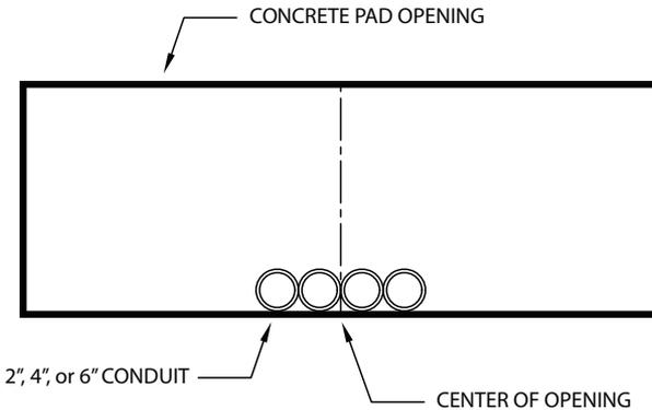
Conduit sizes may vary with design. If conduit number and size are different than as shown, please contact KUA's Conduit Inspector.
