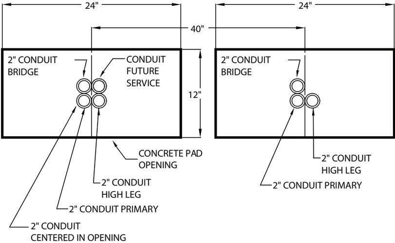
Conduit sizes may vary with design. If conduit number and size are different than as shown, please contact KUA's Conduit Inspector.
