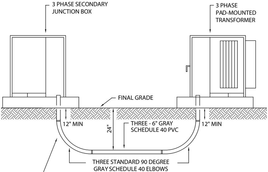
ADDITIONAL DEPTH IS REQUIRED FOR PLACEMENT OF LONG SWEEP 90 DEGREE ELBOWS.
