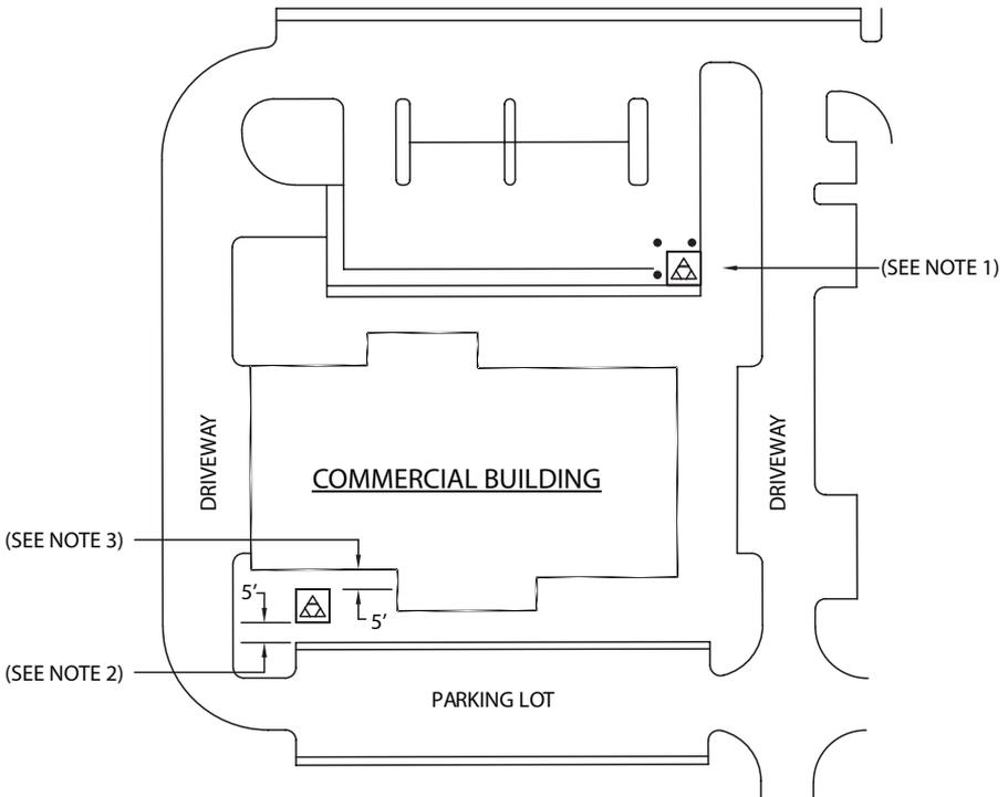
Protection of Transformers and Junction Boxes: The transformer and/or junction box shall be protected by the following means:
