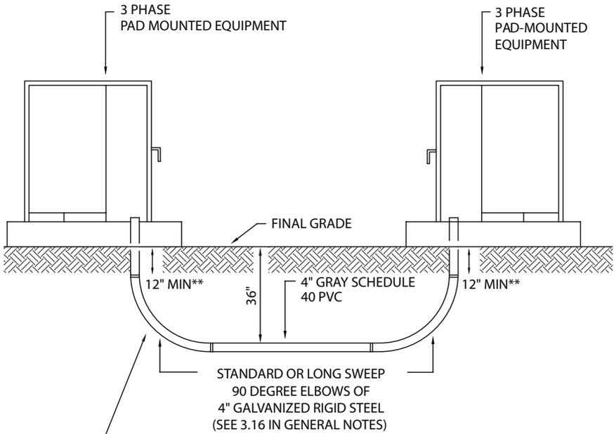
ADDITIONAL DEPTH IS REQUIRED FOR PLACEMENT OF LONG SWEEP 90 DEGREE ELBOWS.
