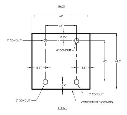
Type 13 and 14 Switchgear Conduit Stub-up Layout
