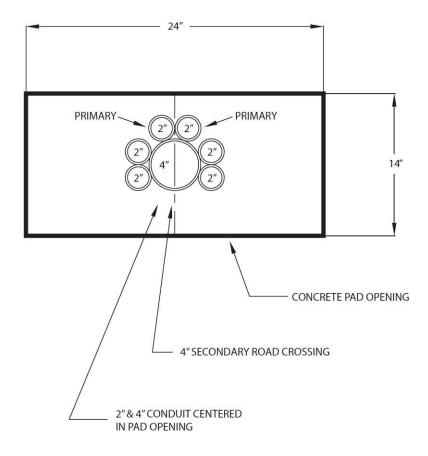
Single Phase Transformer (167 or 250kVA) Conduit Stub-up Layout
