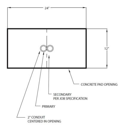
Three Phase Transformer Conduit Stub-up Layout (500kVA or Less)
