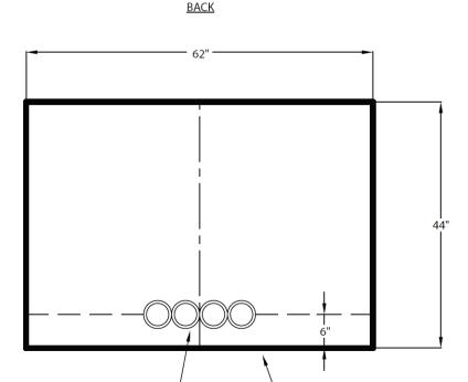
Conduit sizes may vary with design. If conduit number and size are different than as shown, please contact the project Engineer.
