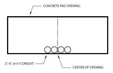
Single Phase Transformer Conduit Stub-up Layout
