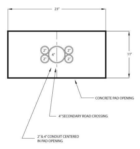
**Primary Junction Box Conduit Stub-up Layout**
