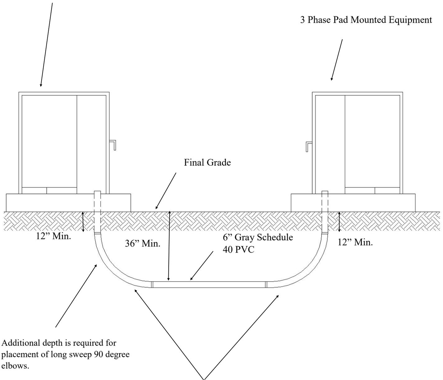
Additional depth is required for placement of long sweep 90 degree elbows.
