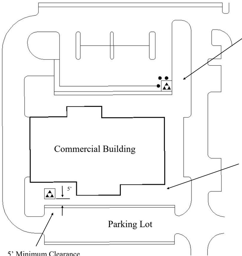
When transformer is located in pavement, 6” iron pipes must be installed. (See Note 1)
