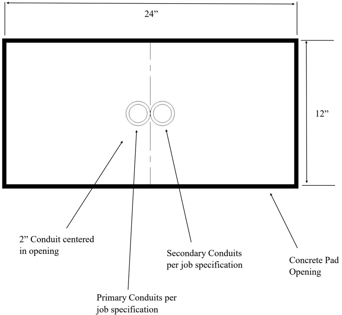
Conduit sizes may vary with design. If conduit number and size are different than as shown, please contact KUA's conduit inspector.
