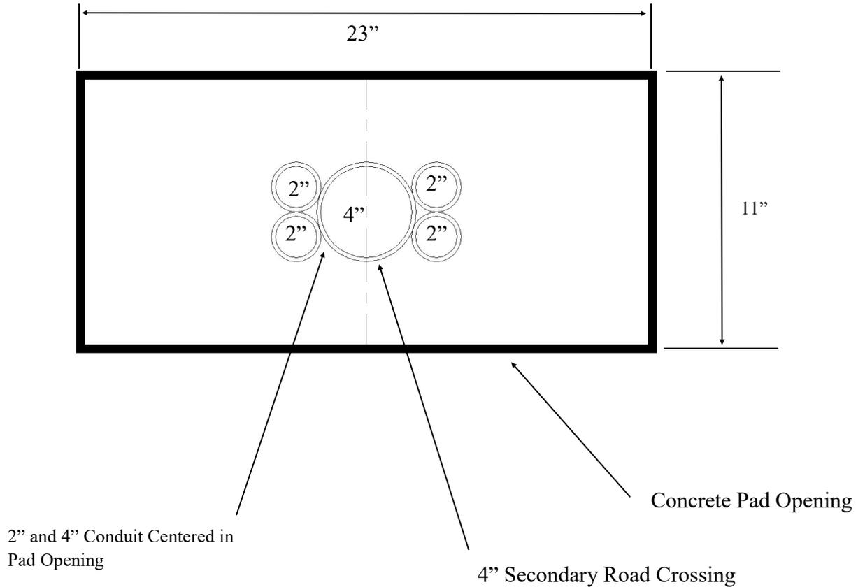
Conduit sizes may vary with design. If conduit number and size are different than shown, please contact KUA's conduit inspector.
