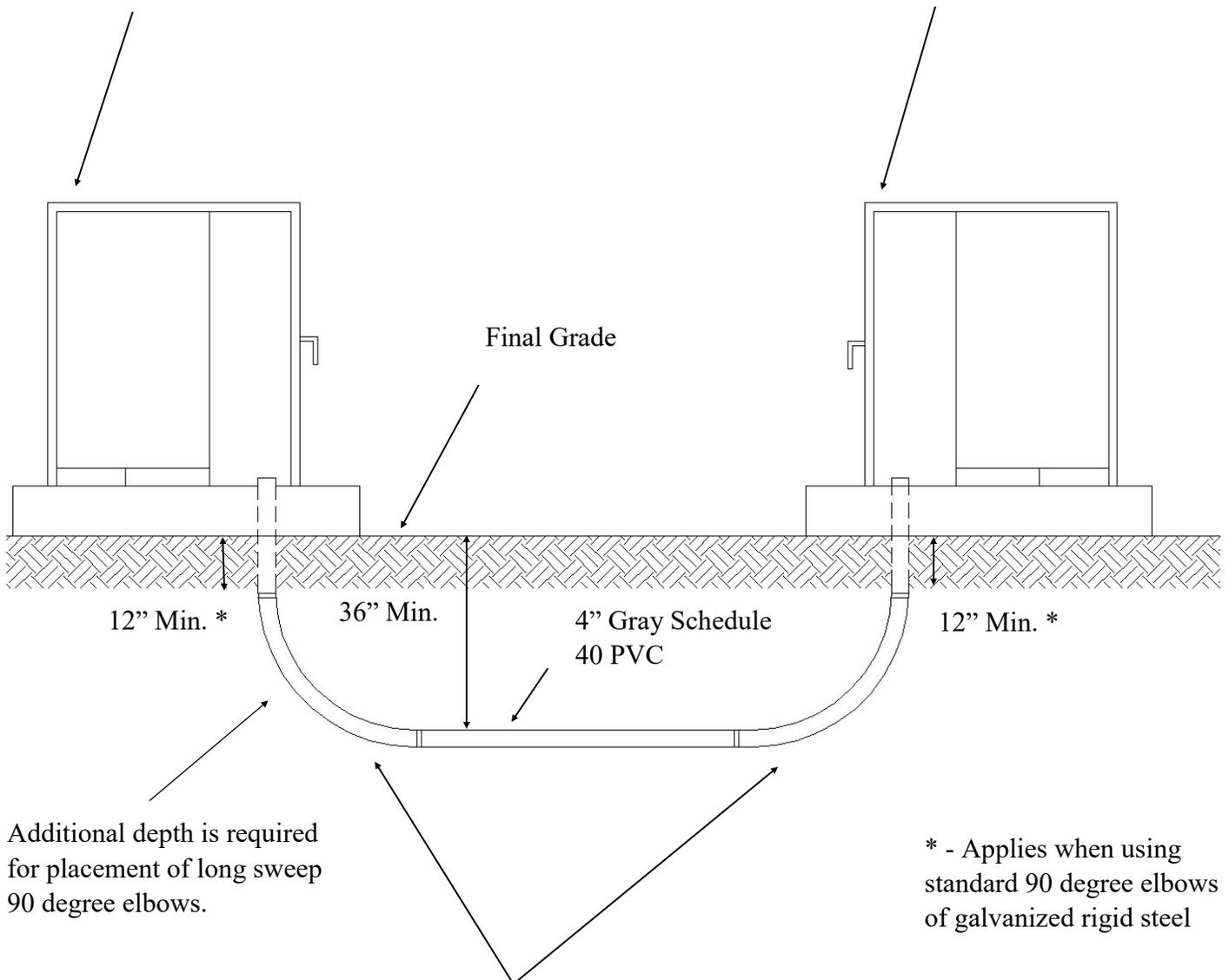
Standard 90 Degree Elbow of 4" Galvanized Rigid Steel (See 3.16 in General Notes)
