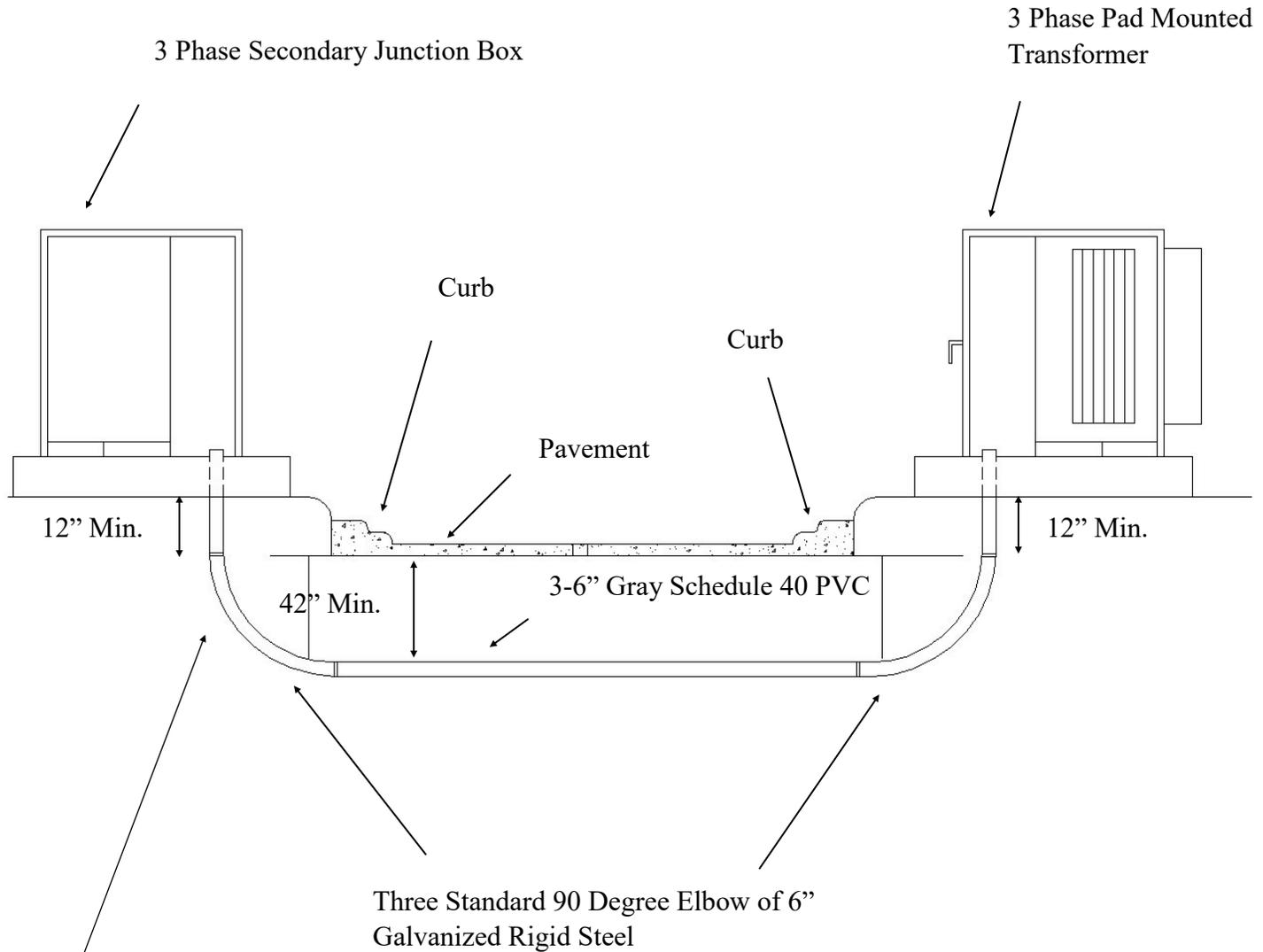
Additional depth is required for placement of long sweep 90 degree elbows.
