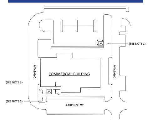
Protection of Transformers and Junction Boxes: The transformer and/or junction box shall be protected by the following means:
