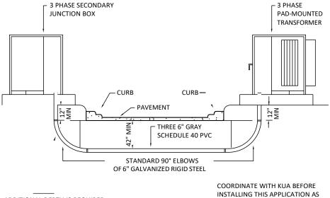
ADDITIONAL DEPTH IS REQUIRED FOR PLACEMENT OF LONG SWEEP 90 DEGREE ELBOWS. COORDINATE WITH KUA BEFORE INSTALLING THIS APPLICATION AS ADDITIONAL REQUIREMENTS MAY BE REQUIRED DEPENDING ON PROJECT CONDITIONS.
