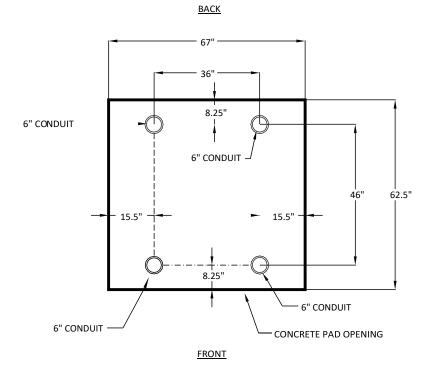
Conduit sizes may vary with design. If conduit number and size are different than as shown, please contact KUA's Conduit Inspector.
