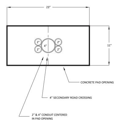
**Primary Junction Box Conduit Stub-up Layout**
