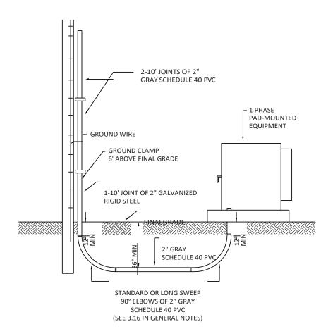
3 Phase Primary Underground Conduit for Conductors 4/0 or Greater
