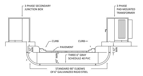
ADDITIONAL DEPTH IS REQUIRED FOR PLACEMENT OF LONG SWEEP 90 DEGREE ELBOWS.
