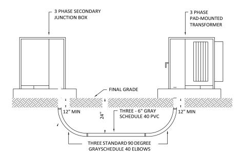
ADDITIONAL DEPTH IS REQUIRED FOR PLACEMENT OF LONG SWEEP 90 DEGREE ELBOWS.
