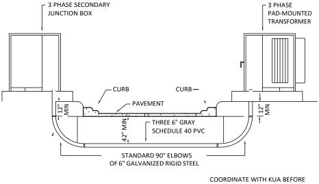
ADDITIONAL DEPTH IS REQUIRED FOR PLACEMENT OF LONG SWEEP 90 DEGREE ELBOWS. COORDINATE WITH KUA BEFORE INSTALLING THIS APPLICATION AS ADDITIONAL REQUIREMENTS MAY BE REQUIRED DEPENDING ON PROJECT CONDITIONS.
