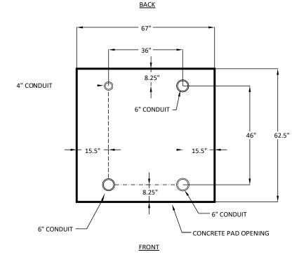
Conduit sizes may vary with design. If conduit number and size are different than as shown, please contact the project Engineer.
